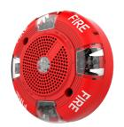
· All strobe appliances have two wiring terminals that accept two #12 to #18 American Wire Gauge (AWG) wires at each screw terminal. Strip leads 3/8 inches and connect to screw terminals.
